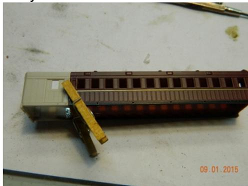
Step 4 : **This is the IMPORTANT part If you do this to the wrong end you have stuffed it.** Modifying the floor, all modifications are done to the END with the REMOVABLE BOLSTER. The right hand end in the photo below. The first step is to remove Bogies, coupler and the buffers and set aside. The buffers just pull out. As per photo below. Next you will need to trim the 2 sets of steps off flush with the floor. I used a saw mounted in a knife handle.
